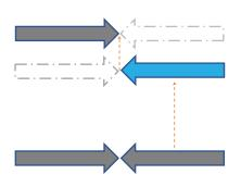
An option on the new SMT-II is "Follow-Me". If your SMT process is not being controlled by Hermes, this independent auto width change system continually monitors the moving rail on the machine before or after the SMT-II. During board change overs this feature removes the need for the operator to be involved increasing process up-time.
